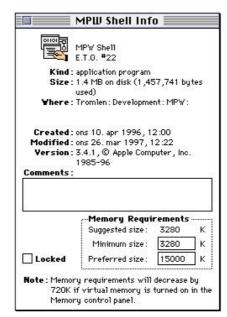
More memory allocated to  ${\tt MPW}$  makes the compiler and especially the linker run faster.
