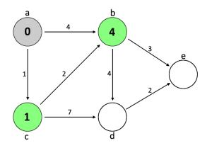
Figure 6: The nodes as they look after the first iteration of Dijkstra's algorithm.
