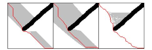
Figure 11: A\*s behavior using different heuristics. Move distance (left); Euclidean distance (Middle); Manhattan distance (Right). The found path is marked in red, while explored nodes are marked in grey.
