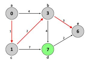
Figure 9: The fourth and final iteration of Dijkstra's algorithm.
