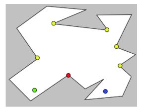
Figure 28: We want to find a path from the green node to the blue node, and we have just arrived at the red node. Because of Property One, we can at this point ignore all the protruding corners marked in yellow.
