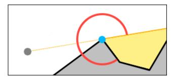
Figure 32: If we at some point have to search for successor points, we can use our preceding position (grey dot) to limit the area in which we have to search (we only have to search the yellow area). This leads to an even earlier early termination, when used in combination with a BSP.
