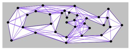
Figure 23: A polygonal world, with its visibility graph, consisting of nodes and edges.
