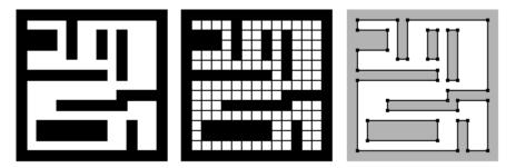
Figure 35: An example of a simple black and white image that is converted into a grid map and a polygonal map.
