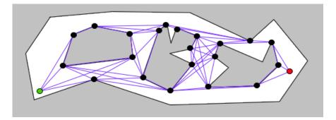
Figure 25: The start and goal nodes are added to the graph at runtime.
