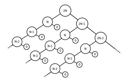
Figure 34: The worst case BSP tree created by the line segments from figure 23. The number of line segments to consider at each recursive call in the construction of the BSP tree is written inside the nodes.
