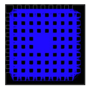
Figure 47: The visibility graph created by VG (Edges marked blue).
