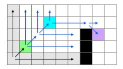
Figure 18: A node (green) is searching diagonally for successors. A successor node (blue) is found, since it is in line of sight of another node, which has a forced neighbor (purple).
