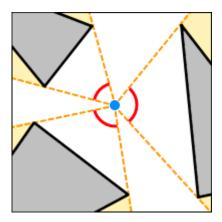
Figure 31: A point marked in blue from which we want to calculate visibility. So far the BSP has returned the three closest line segments, which means that certain angular intervals of our view field are blocked (marked in red).
