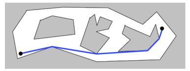
Figure 5: The shortest path from one point to another in a polygonal world.
