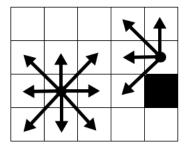
Figure 1: A small 8-connected grid map with one obstacle cell.
