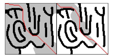
Figure 12: The same pathfinding problem in an 8-connected grid world using Dijkstras algorithm (left) and A\* (right). The path is marked in red, and the explored nodes are marked in grey. The start node is in the top left corner and the goal in the bottom right corner.
