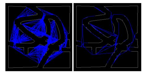
Figure 30: On the left we see the visibility graph used by the VG algorithm (VG). On the right we see what is left of this visibility graph after we have applied property one (VGO).
