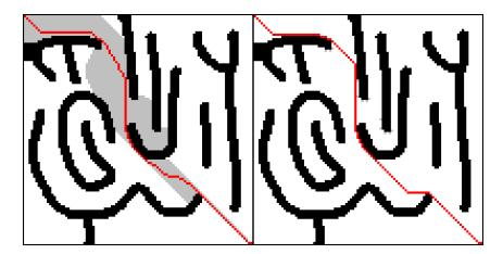
Figure 19: A\* (left) compared to JPS (right), with explored nodes marked in grey.
