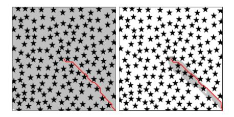
Figure 40: Explored areas are marked in grey. Dijkstra (left) explores significantly more grid cells than A\* (right), before a path is found from the center to the bottom right corner.
