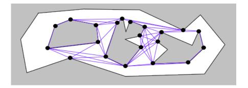
Figure 24: The visibility graph used in the context of pathfinding.
