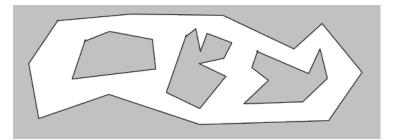
Figure 3: A polygonal world, with obstacles marked in grey, and a traversable area marked in white.
