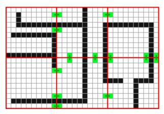
Figure 21: Node pairs at each entrance is marked.
