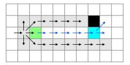
Figure 14: In this figure we want to find successors of the green node.
