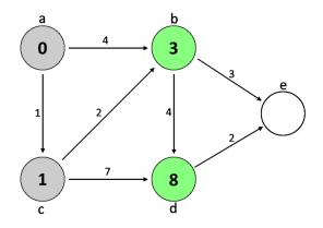
Figure 7: The second iteration of Dijkstra's algorithm.
