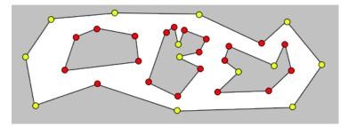
Figure 4: A polygonal world with protruding corners (red) and depressed corners (yellow).
