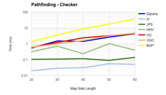
Figure 48: Results from pathfinding in the Checker map.
