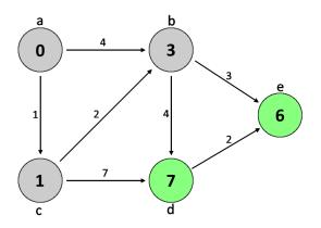
Figure 8: The third iteration of Dijkstra's algorithm.
