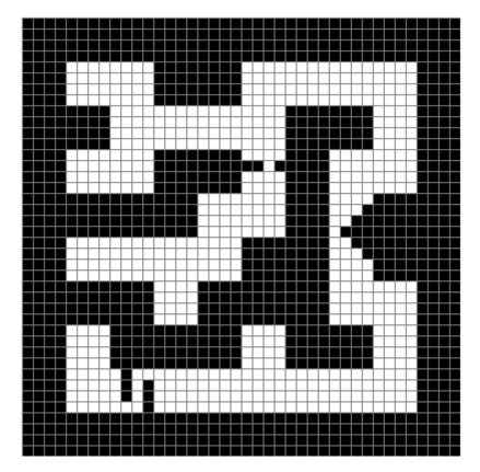
Figure 56: An example of a map with a varying level of detail. Most of the corridors are of the same width, however the grid cell resolution cannot be lowered without sacrificing detail.
